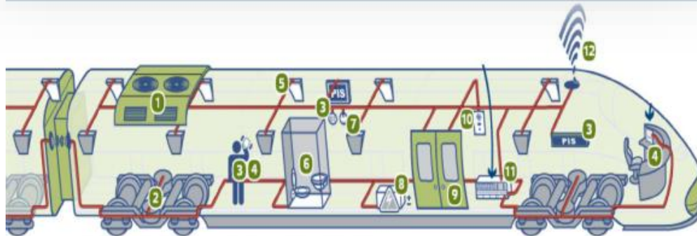
TRAINNET™ TCMS, FOR THE MONITORING, CONTROL AND AUTOMATION OF:
