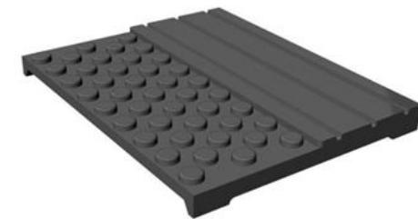
Structural design model of stiffness partitioning on the left and right sides of the rail pad
