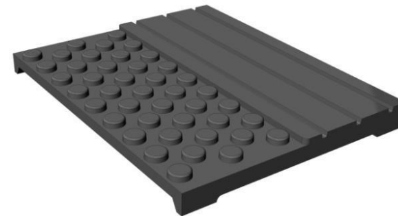
Structural design model of stiffness partitioning on the left and right sides of the rail pad
