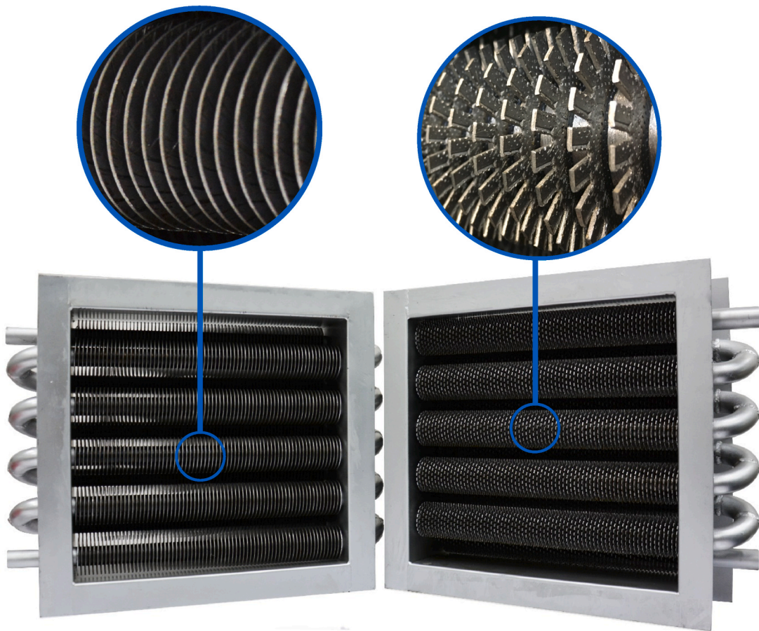
Fig. 4. The tested plain welded spiral fin-and-tube heat exchanger (left) and serrated welded spiral fin-and-tube heat exchanger (right).
