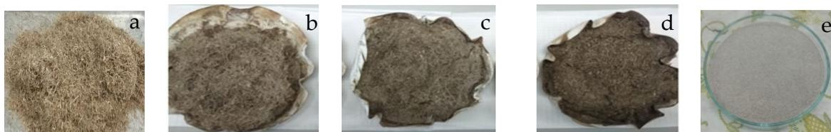
**Figure 1.** Appearance comparison of (a) untreated SCT, (b) pretreated SCT at 140 °C, (c) pretreated SCT at 160 °C, (d) pretreated SCT at 180 °C and (e) pretreated and bleached SCT (PB-SCT).
