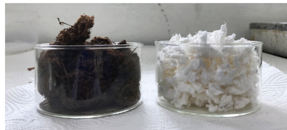
Fig. 1 – Appearance of the bamboo fibers after the steam explosion (left) and the combined steam explosion and chemical treatments (right).
