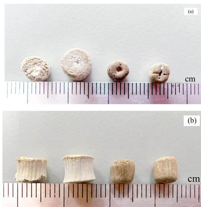
Figure 2. Top-view (a) and side-view (b) photographs of Lead tree wood-zeolite composites of (from left to right) untreated wood (NR), untreated wood with sonication (NRS), refluxed wood (R) and refluxed wood with sonication (RS).
