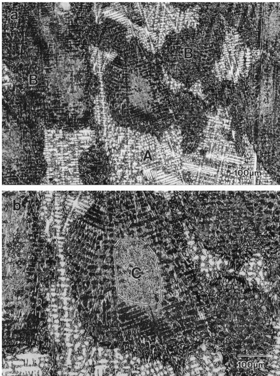
**Fig. 2.** (a) General microstructure from upper region of test bar. Areas of dendritic austenite plus eutectic  $M_7C_3$  carbides are indicated as (A) whilst the dendritic matrix of ferrite and carbide precipitates (darker etching) are marked (B). (b) This view shows an apparent dendrite free zone at the core of a ferrite area, marked (C). Optical view: Etchant is 50 mL of HCl and 10 g of  $Na_2S_2O_3$  in 100 mL distilled water.
