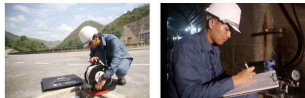
Fig. 4. Manual measurements and recording: ground water level (left); pressure gauge (right).
