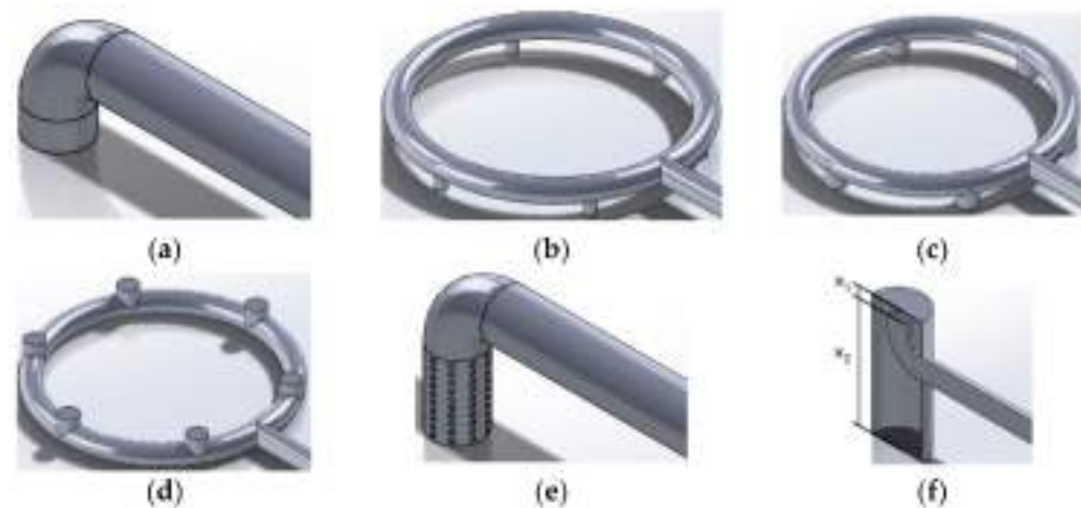
Figure 3. The geometries of the modified inlet pipes: (a) Direct downward model; (b) Annular inlet I model; (c) Annular inlet II model; (d) Annular inlet III model; (e) Perforated pipe model; (f) Equalizer I-IV models.
