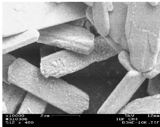
Fig. 5. Surface structure of reacted \text{Bi}_2\text{Ti}_4\text{O}_{11} crystals with excessive \text{Na}_2\text{CO}_3 .
