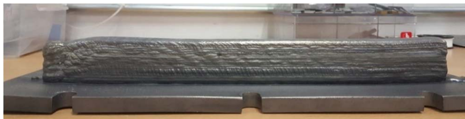
Figure 5. Photographs of the deposited walls: 20 layers.
