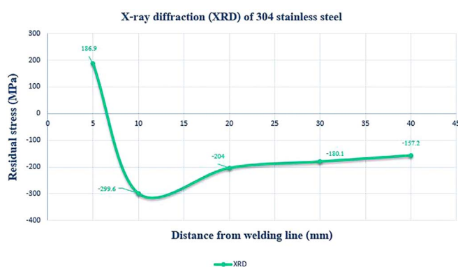
Figure 18. The residual stress result by XRD (304 stainless steel).
