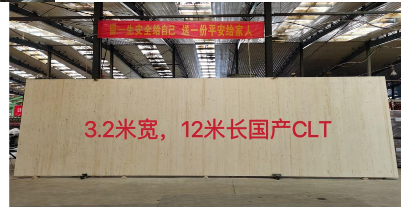
CLT panel with length of 12 m and width of 3.2 m
