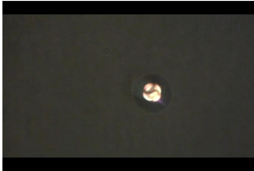
Lehmann rotation of defect on liquid crystal droplet inclusions due to heat gradient
