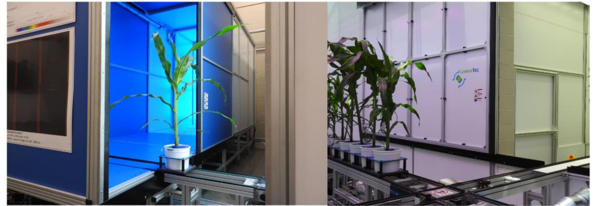
LemnaTec Scanalyzer 3D high-throughput plant phenotyping facility at the UNL : view of the automated greenhouse ( top-left ); watering station ( top-right ); a plant entering the fluorescent chamber ( bottom-left ); and plants on the conveyor belt heading towards the visible light chamber ( bottom-right ).
