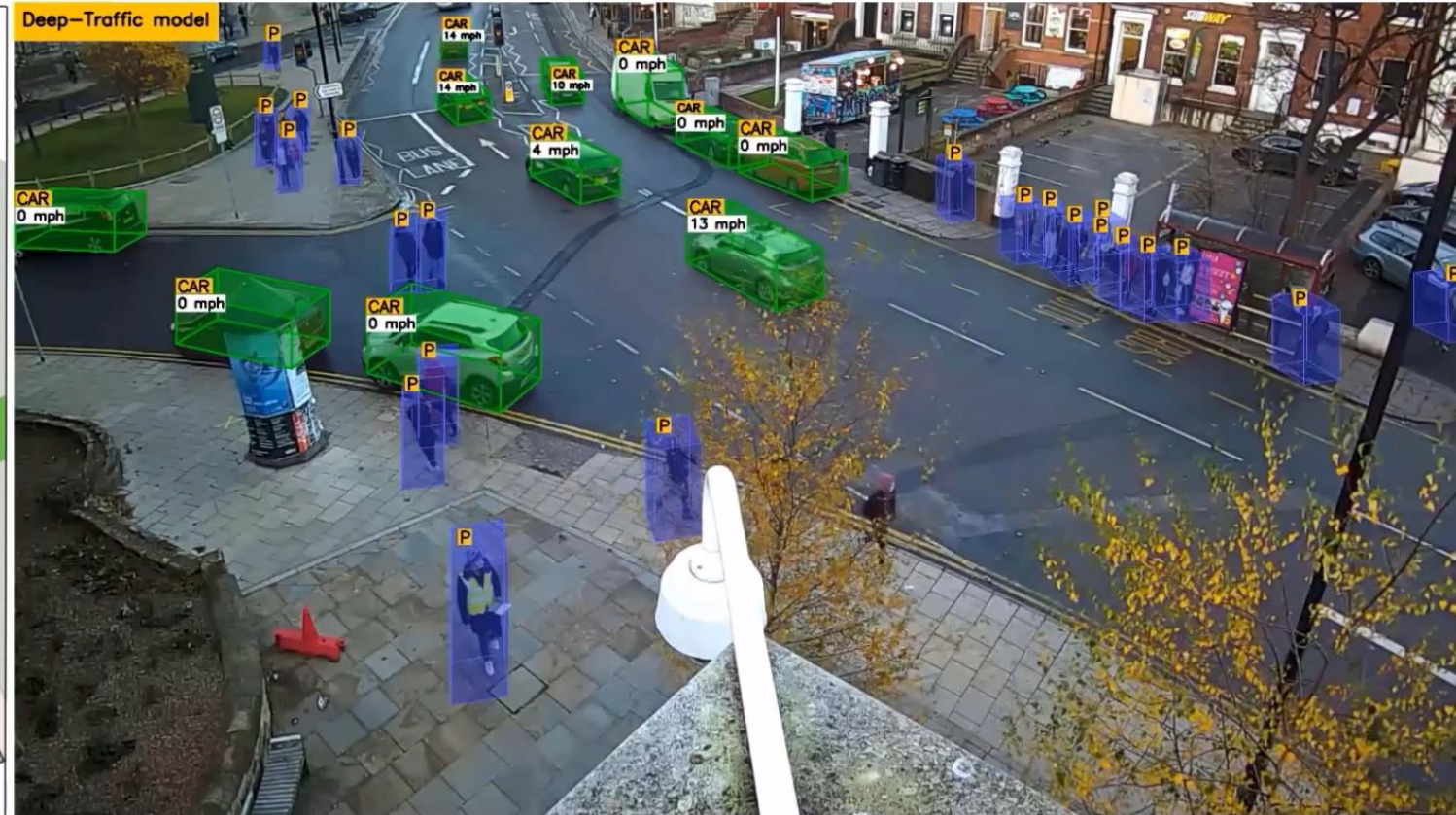
3D bounding boxes, speed detection, and angular trajectory estimation
