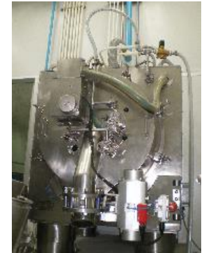
Isolation / Filtration unit
