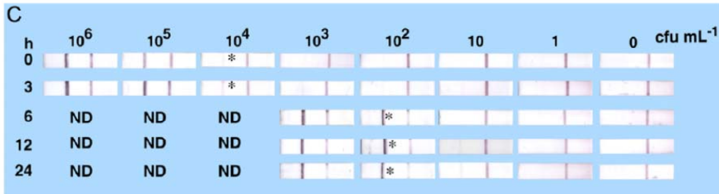
Fig. 5. Detection sensitivity of the strip test after pre-enrichment in shrimp homogenate in APW. A similar experiment was performed using shrimp homogenate in APW (1:10=weight:volume) as diluents. * represents the lowest detection limit.
