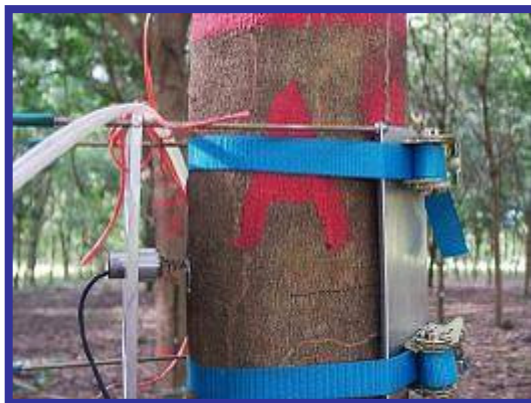
Linear Variable Displacement Transducer, LVDT
