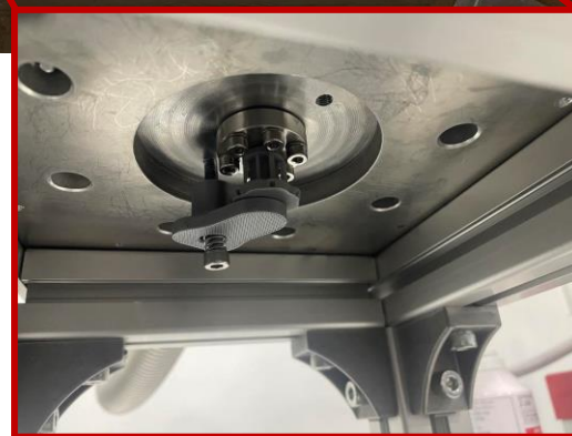
Sample holder was placed at the electron gun exit.
