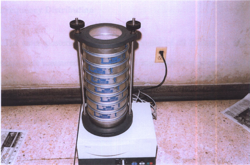
Figure 14 The Shaking Sieve for Grain Size Analysis
