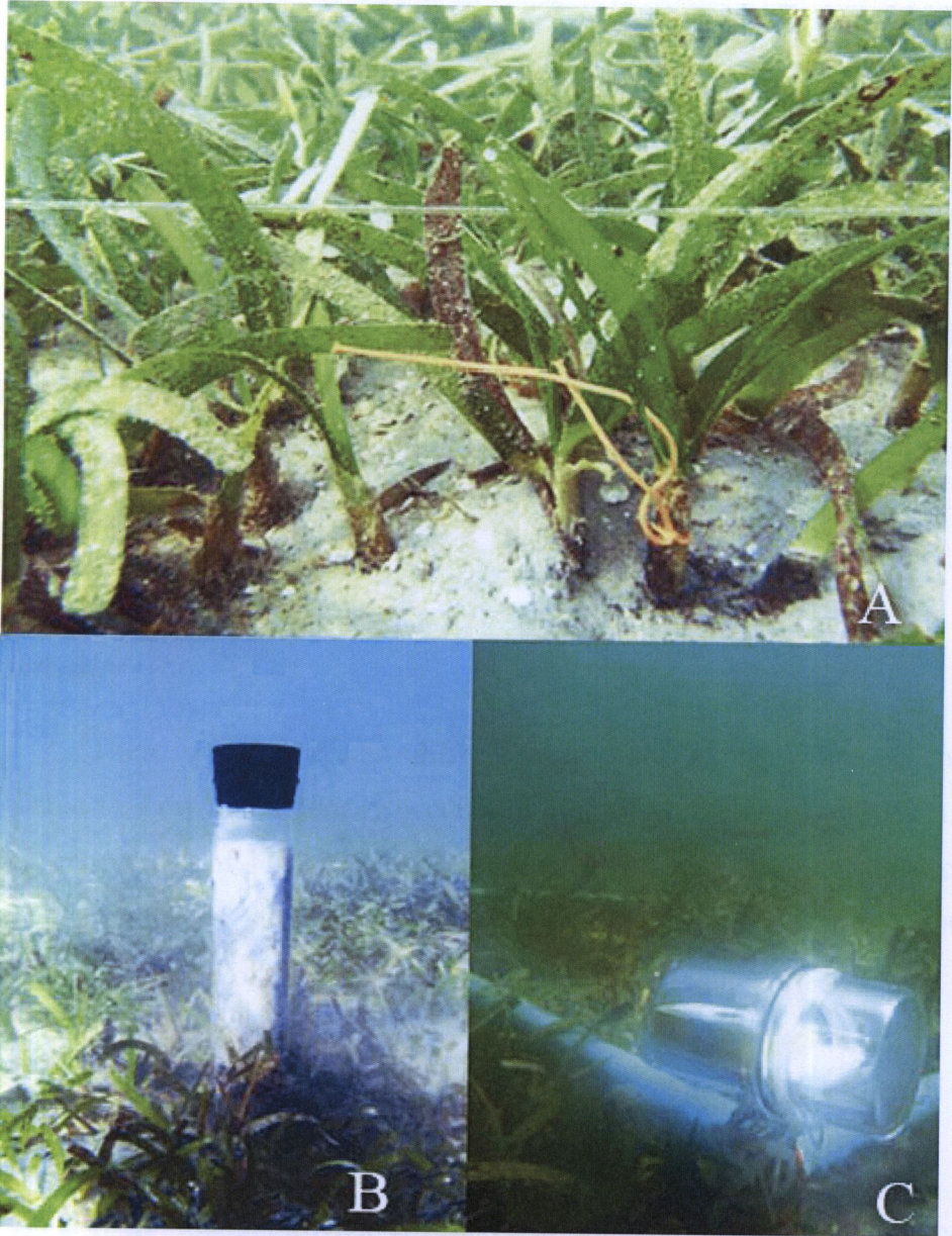
Figure 8. Field set up: A. Plant was punched and marked with a string, B. Sediment was collected by plastic core for nutrients in the sediment analysis, C. Data logger set on the permanent plot at the same height of the T. hemprichii tip, about 10 cm from substrate.
