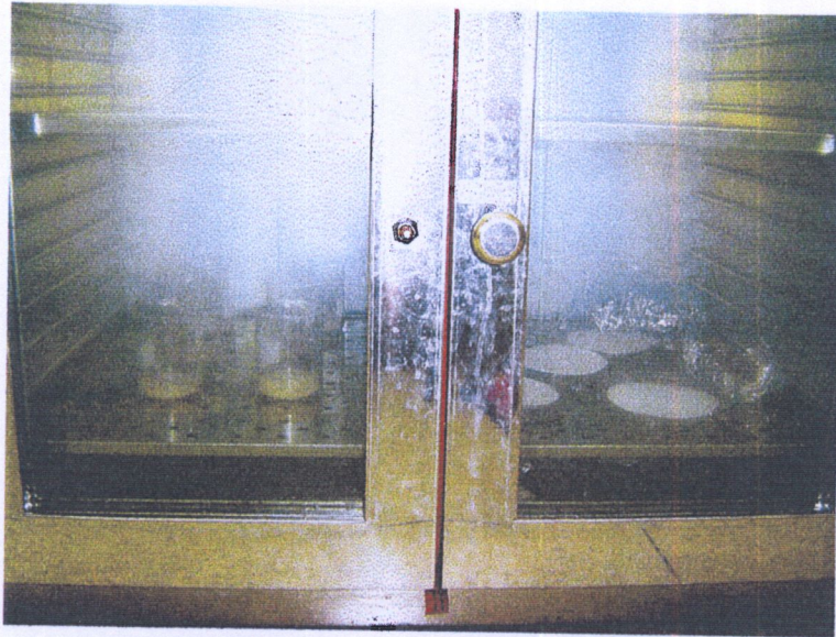
Figure 8 Dry sediment from a sediment trap at 105°C, 24 hour
