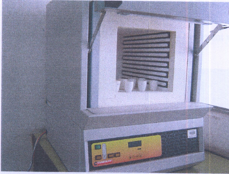
Figure 10 Dry sample burn in muffle furnace at 550°C, 5 hours to remove organic matter
