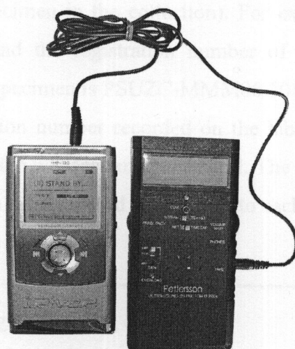
Figure 14. Pettersson ultrasound detector D 240x in time-expansion (10x) mode, connected to sound recorder i-RIVER model: iHP-120 Multi-codec jukebox
