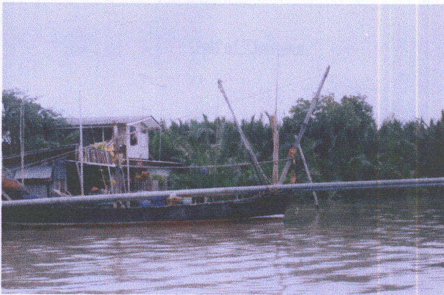
Figure 8. Sampling boat equipped with push net.
