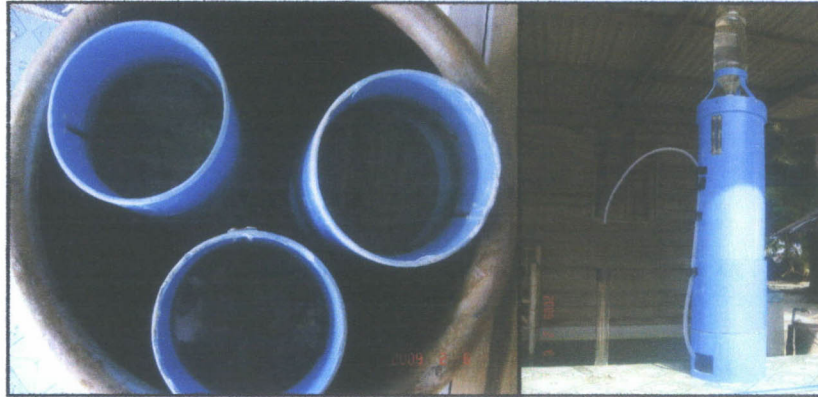
Figure 3-9 Saturated Hydraulic conductivity test of abandoned shrimp pond soil
