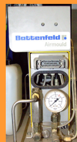
Gas Injection Module
